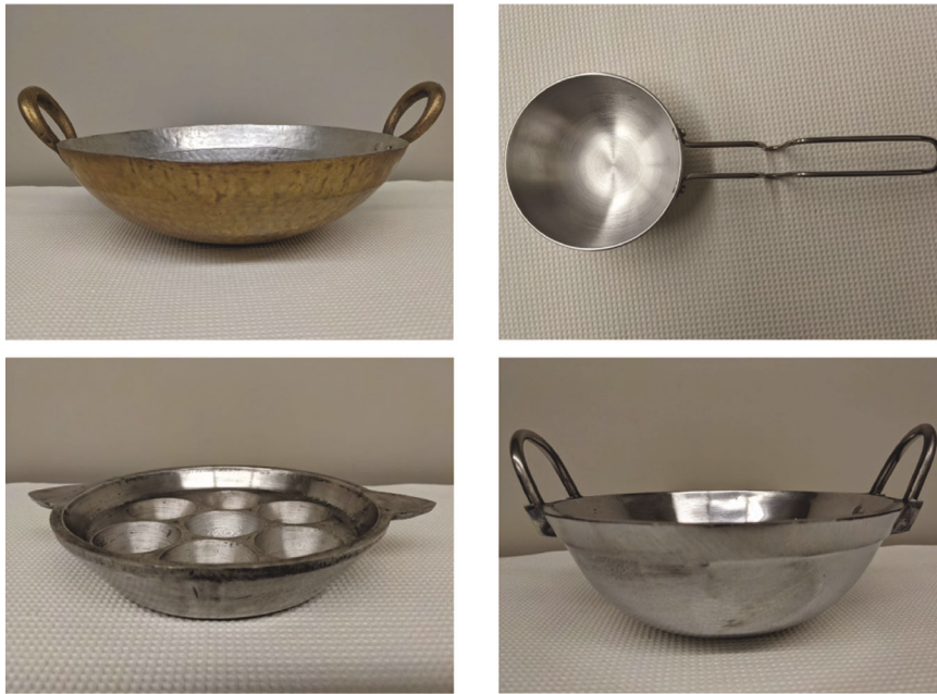
Fig. 1 Examples of Indian cookware purchased for testing. Top left: Brass kadai (Pot #51). Top right: Hindalium/indolium tadka pan (Pot #53). Bottom left: Hindalium/indolium appam pan (Pot #54). Bottom right: Hindalium/indolium kadai (Pot #55).
